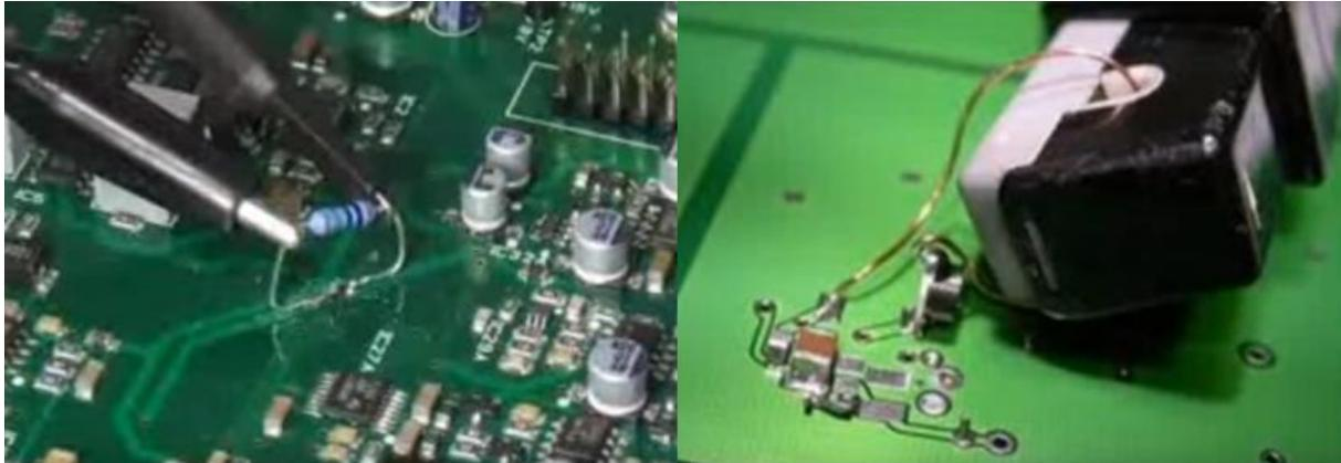
Breaking the circuit and inserting a resistive shunt
