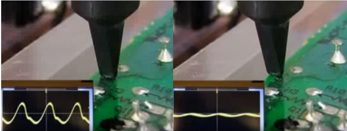
Positioning of the i-Prober to the conductor is critical
