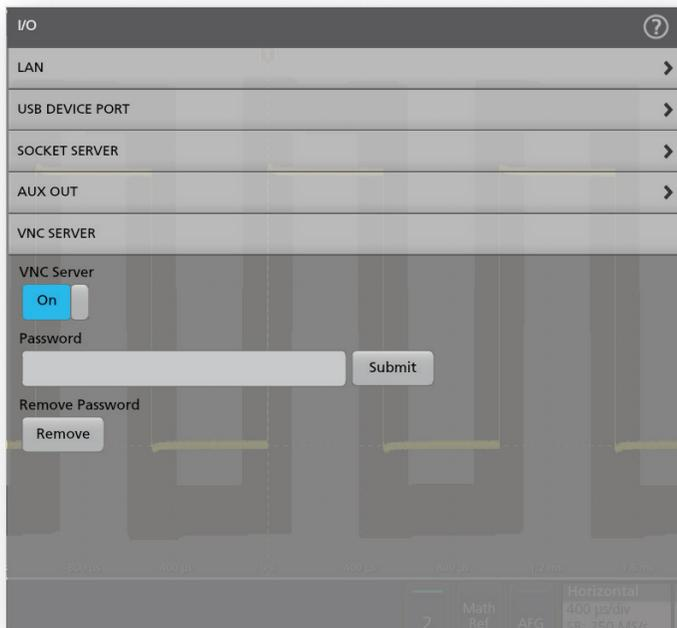
Figure 6: Enabled VNC server on the 2 Series MSO.
