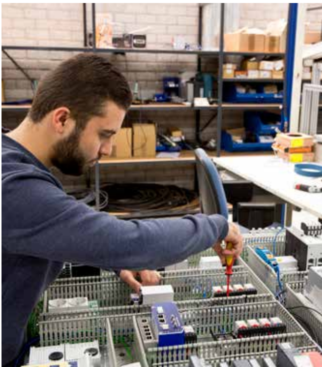
Push-In Plus technology makes the wiring of control panels much easier and faster.
